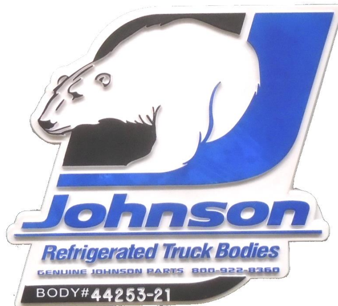
Figure 11: Truck body serial number badge. This serial number is 44253. The -21 year code indicates a 2021 manufacture date. This badge is typically located on the front left corner of the truck body.
