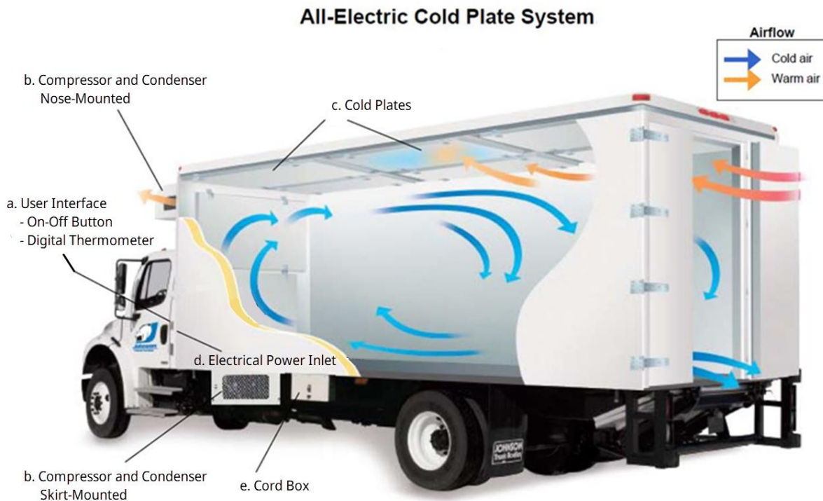
Figure 1: Refrigeration System Diagram
