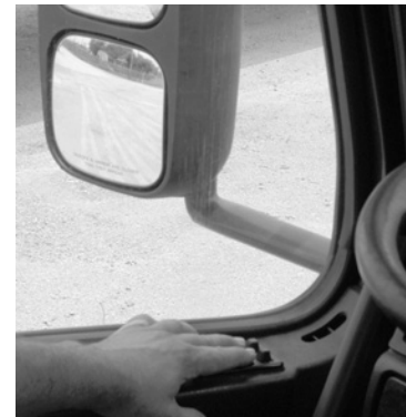
5. See if mirrors on both sides of the cab are clean and aligned.
