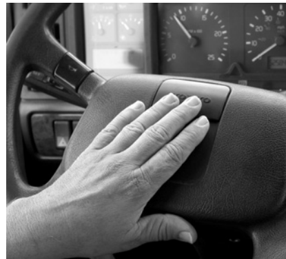
3. Sound the horn, test for excess amount of wheel play.
