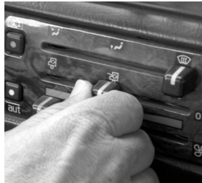
6. Test heater-defroster blower.
