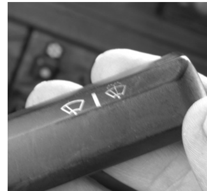
4. Test washer-wiper and examine windshield for cracks.
