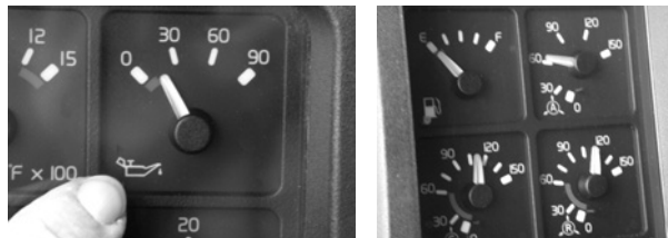
2. Check oil pressure, warning lights, air pressure. Deplete pressure until warning buzzer sounds
