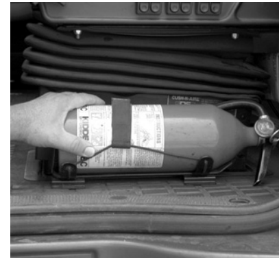
7. Check for charged fire extinguisher and emergency equipment.
