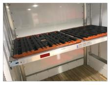
**Double Decking Option** The innovative Double Dex option creates a second deck to accommodate additional cargo by using captive beams within a recessed track.
