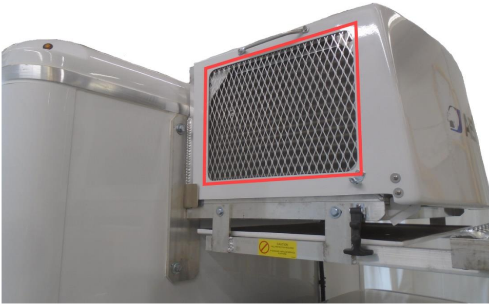
Figure 4: Condenser Coil location on a nose-mounted condensing unit.
