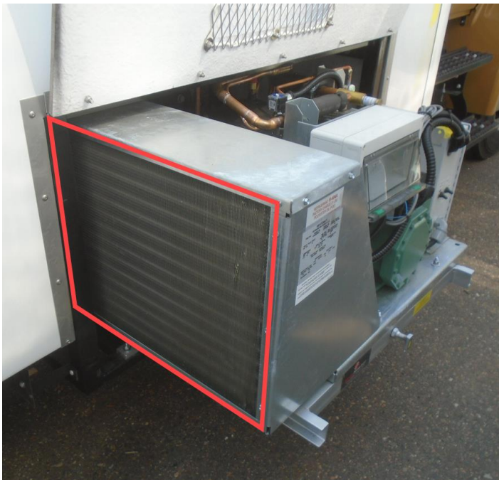
Figure 5: Condenser Coil location on a skirt-mounted condensing unit.
